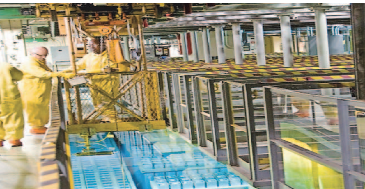
Spent (used) fuel from research reactors around the US and the world is safely stored for processing.
